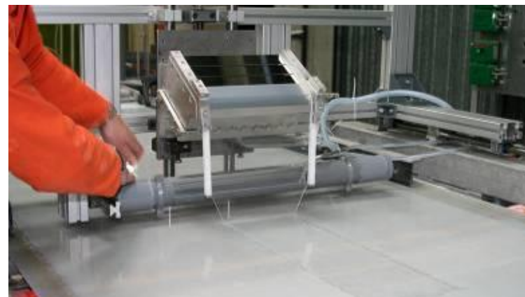
CTP's curtain coater located above Grenoble INP Pagora's paper machine
